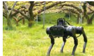
Patrol of a pear orchard by a quadruped robot
