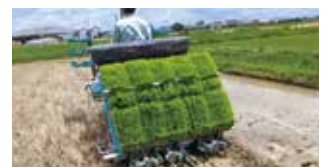
Modification of a commercial rice transplanter for no-till fields aiming at controlling aquatic weeds under no-herbicide condition (Food Resources Education and Research Center)
