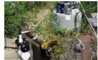
Auto sampler and turbidity meter for water quality observation
